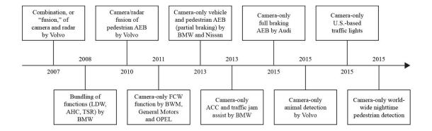
There is a clear trend towards the primacy of the camera sensor. This primacy is driven by the lower cost and packaging benefits of the "bundling effect" of having a single camera performing multiple ADAS and the relative ease of adding functionality through simple software updates. We believe the bundling effect is unique to the camera-based sensing modality since all other sensor modalities specialize in limited ADAS subsets.
