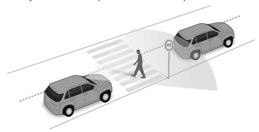
The image above shows some of the detected objects within the 50-degree horizontal field of view of a monocular camera. Integrated with our EyeQ SoC, a monocular camera can detect pedestrians, vehicles, lanes, traffic signs and more.
